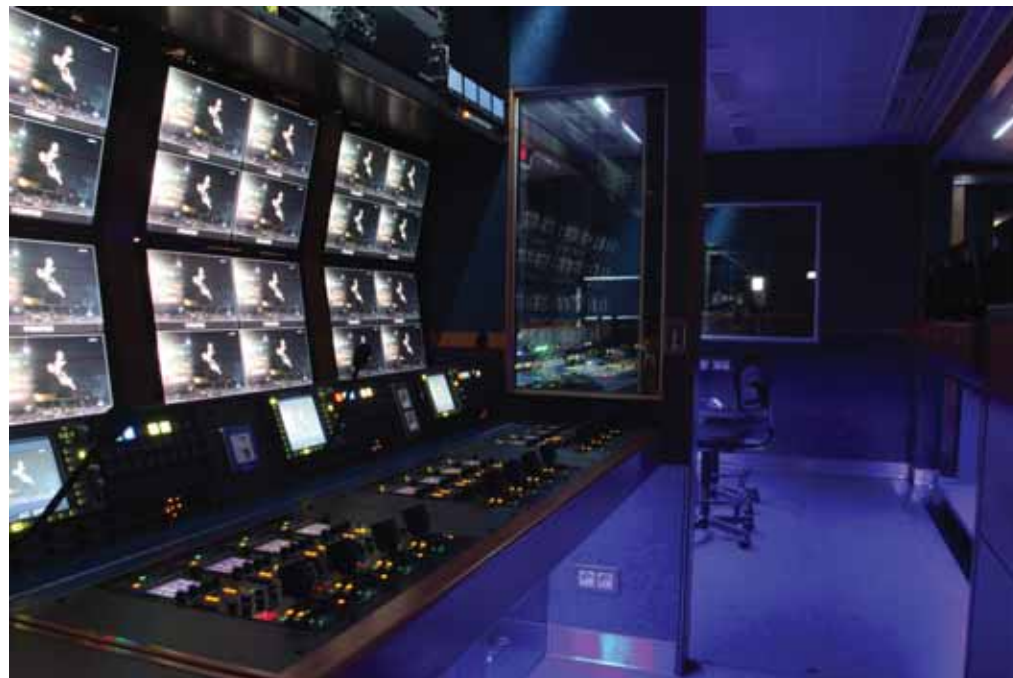
Camera control: Main cameras are mix of HDC-1500R and HDC-3300R, with HDCU-3300 and HDCU-1500 CCUs
